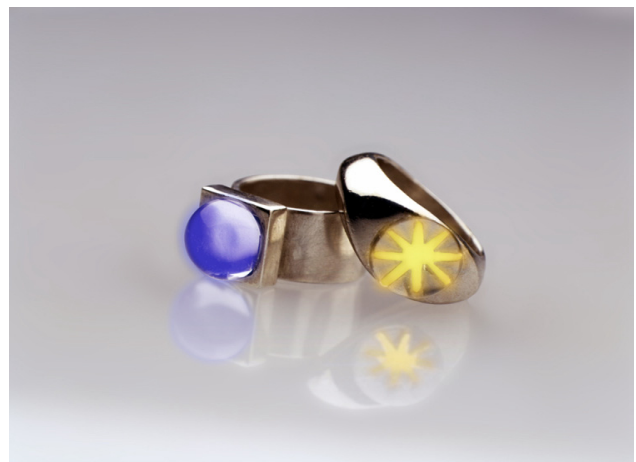
Figure 1: Glowing e-rings with multicolor LEDs can be set to show special colors and sequences of lights when particular events occur. The ring changes state according to messages sent to it from the jewelry server.
